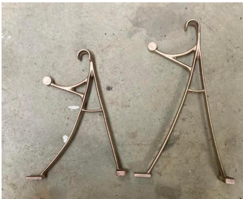
Photo of one the new bellcord support castings.
