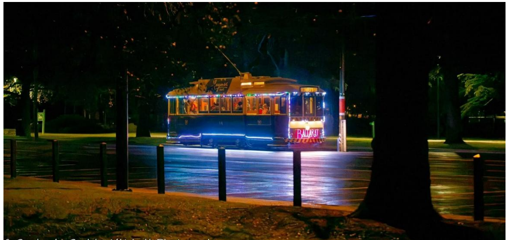
Ballarat tram 14 during the 2026 Winter Festival. The tram has been rewired and low voltage lighting installed. The neon lights are a temporary fitting. Photo Benjamin Boehle Mitchell 25-7-2026
