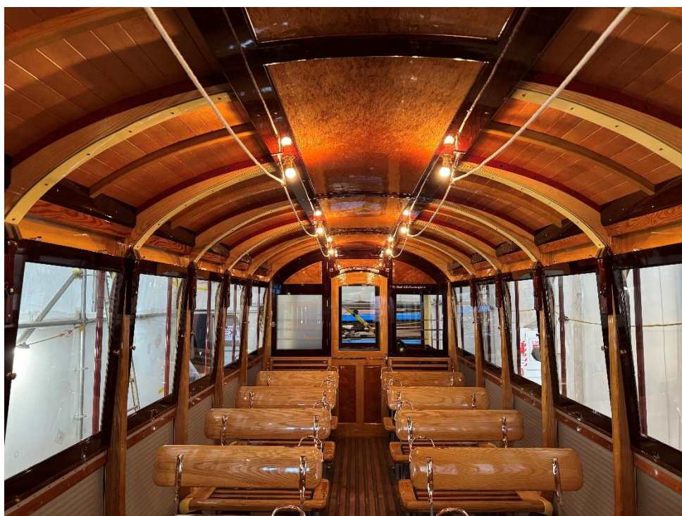
Interior of the tramcar showing the excellent work in the finished tram with the sides closed off to become an enclosed trailer.
